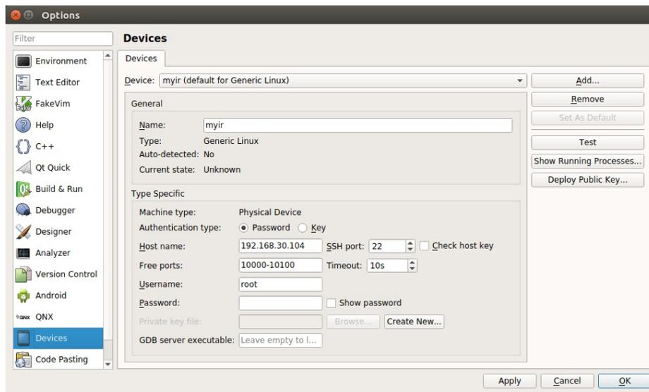
Figure 3-3-1 Device Configuration
