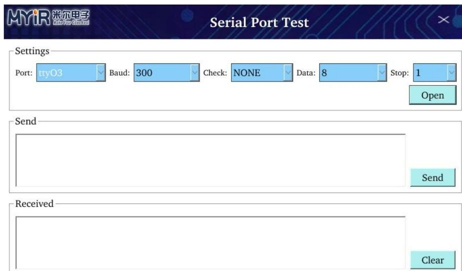
Figure 2-1-1 Local serial port test UI
