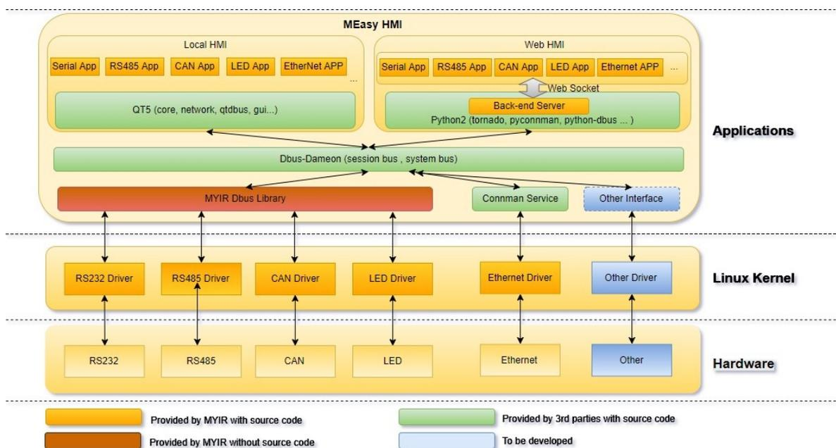
Figure 1-1 MEasy HMI Framework
