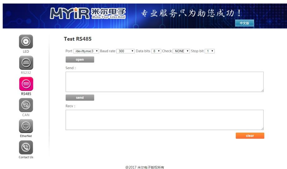
Figure4-2-1 Web HMI Test RS485
