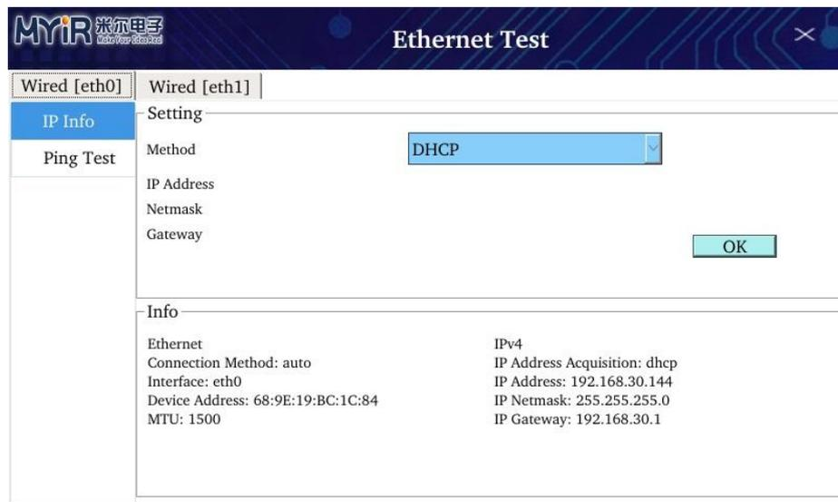
Figure 2-3-1 Development board network port configuration
