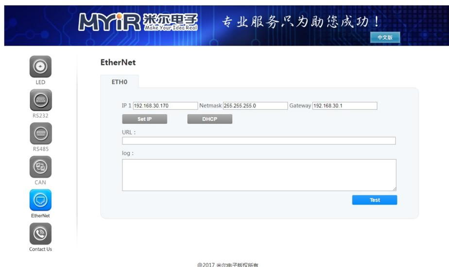
Figure4-3-1 Web HMI EtherNet
